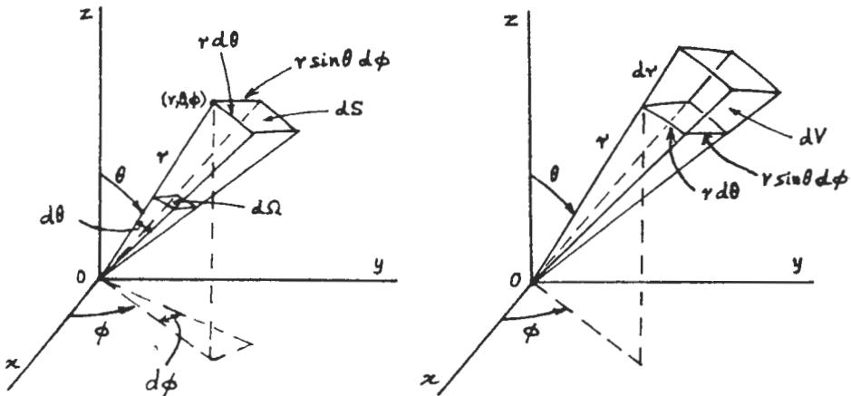
$$dS = r^2 \sin\theta \, d\theta \, d\phi \quad d\Omega = \sin\theta \, d\theta \, d\phi \quad dV = r^2 \sin\theta \, d\theta \, d\phi \, dr$$
