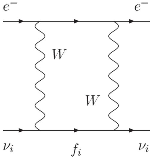
$$\langle r_{\nu_i}^2 \rangle = \frac{G_F}{4\sqrt{2}\pi^2} \left[ 3 - 2 \log \left( \frac{m_i^2}{m_W^2} \right) \right] \quad i = e, \mu, \tau$$
