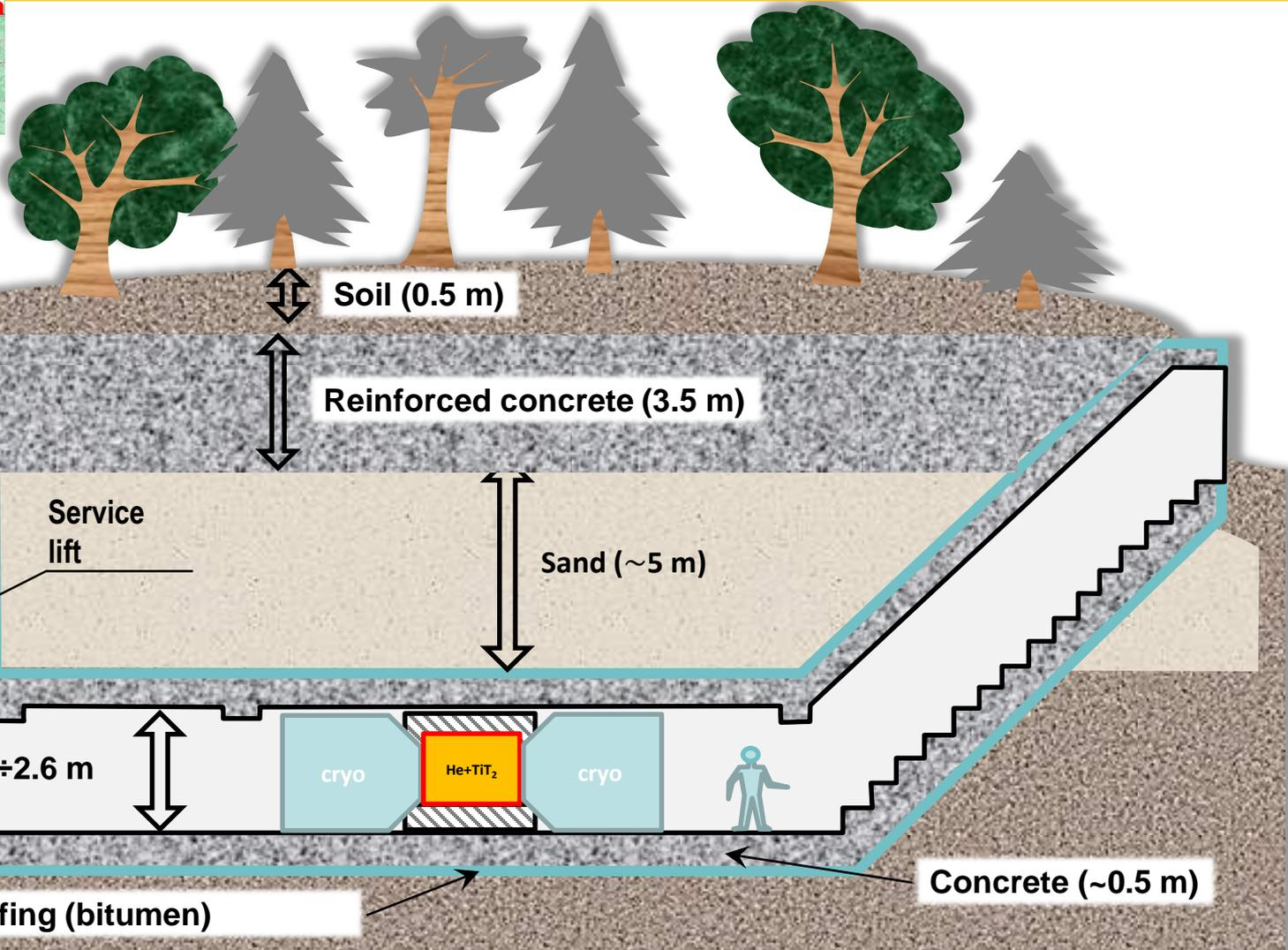
**The overburden of ~18 m.w.e. stops the soft and hadronic components of cosmic radiation**
