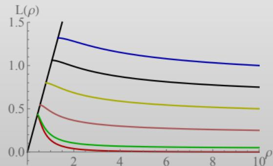
$N_c = 3, N_f = 2, \mu = \sqrt{\rho^2 + L^2}$ ; the  $L(\rho)$  with a massless UV quark has  $L_{IR} = 0.43$ ; quark masses from top to bottom: 1, 0.75, 0.5, 0.25, 0.05, 0. Here units are set by  $\alpha(\rho = 1) = 0.65$ .
