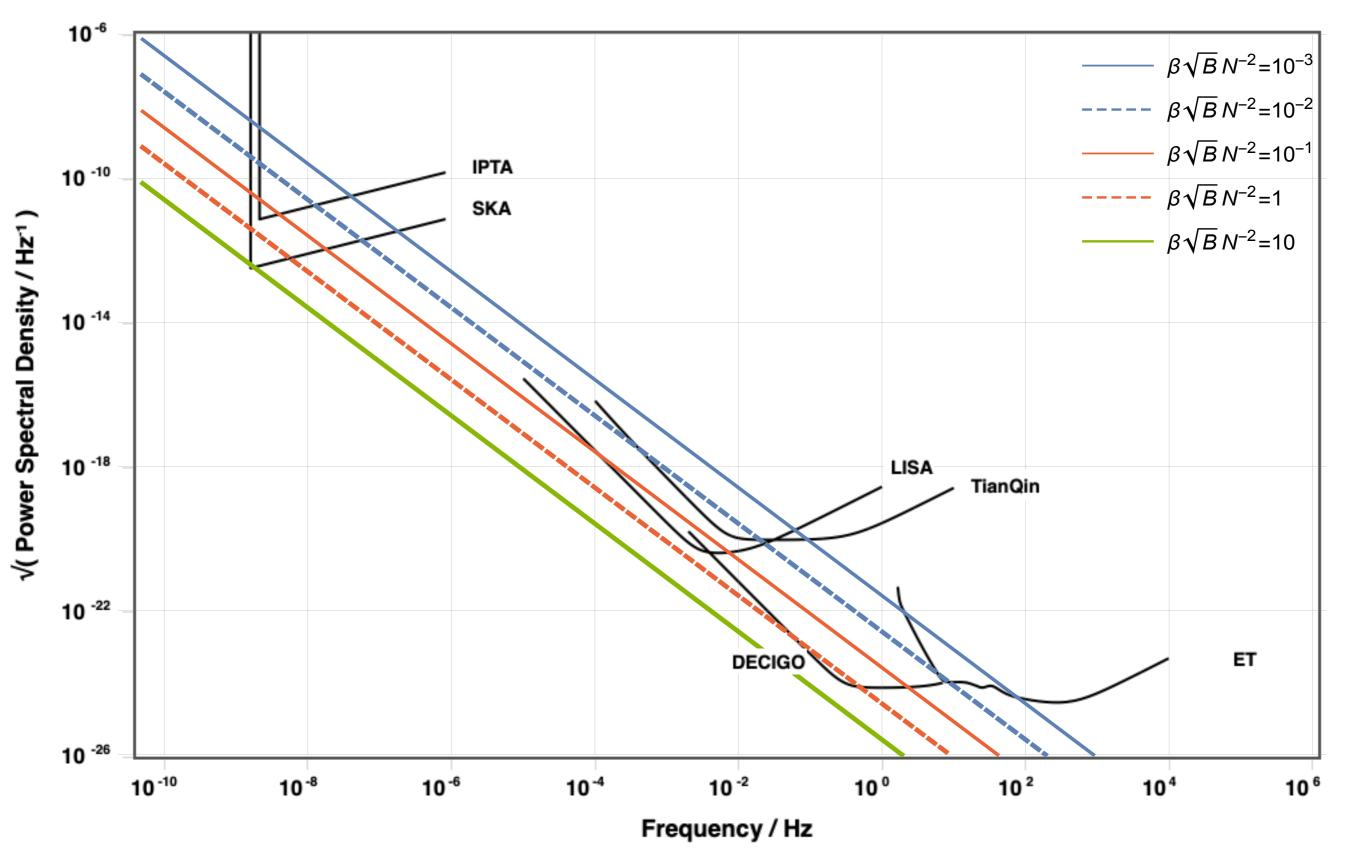
Strain as a function of peak frequency.  $\beta \simeq 1-10$ ,  $B \simeq 1-100$ , N=4-24. One point on each colored line corresponds to a particular set of the parameters of the model and it represents the strain at the peak frequency. Not the spectrum!
