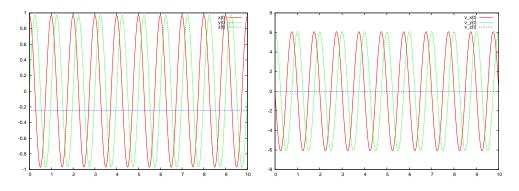
Figure 2.13: The plots of the functions  $x(t), y(t), z(t), v_x(t), v_y(t), v_z(t)$  of the program ConicalPendulum.f90 for  $\omega = 6.28$ , l = 1.0.
