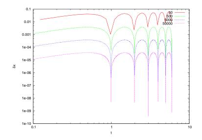
Figure 4.12: Like in figure 4.11 for the Euler-Cromer method. The error becomes approximately ten times smaller each time according to the expectation of being of order  $\sim O(\Delta t)$ .
