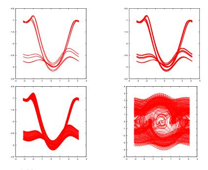
Figure 4.28: A phase space trajectory of the forced damped pendulum. The parameters chosen are  $\omega_0 = 1.0$ ,  $\omega = 2.0$ ,  $\gamma = 0.2$  and A = 1.031, 1.033, 1.04, 1.4. We observe the chaotic behavior of the system.
