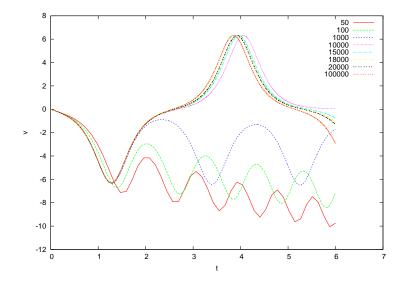
Figure 4.5: Convergence of Euler's method for the simple pendulum like in figure 4.2 for  $\theta_0 = 3.0$ ,  $\omega_0 = 0.0$ . The behavior of the angular velocity is shown and we notice unstable behavior for Nt $\leq 1,000$ .
