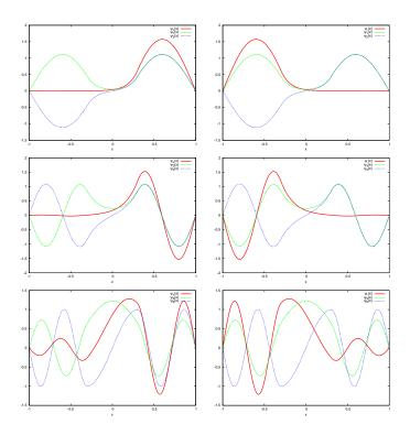
Figure 10.4: The functions  $\psi_{\pm}(x) = (1/\sqrt{2})(\psi_n(x) \pm \psi_{n+1}(x))$  for n = 1, 3, 5 for the double well potential (equation (10.27) with  $v_0 = 100, a = 0.3$ ) are plotted using bold red lines. We observe that the more degenerate the states, the stronger the localization of the particle to the left or right well. The other plots are those of the energy eigenfunctions for n = 1, 2, 3, 4, 5, 6.
