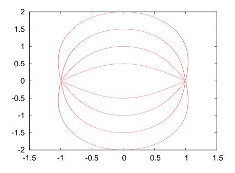
Figure 7.2: Some electric field lines of the electric field of two opposite charges calculated by the program ELines.f90 (version 1!).
