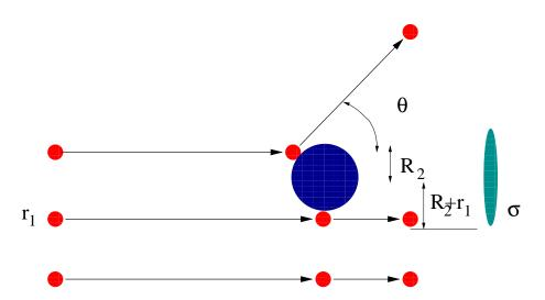
Figure 5.8: Scattering of hard spheres. The scattering angle is  $\theta$ . The cross sectional area  $\sigma$  is shown to the right.
