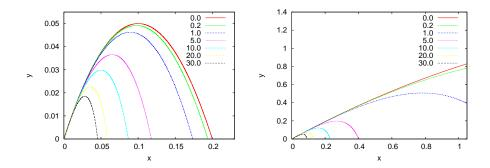
Figure 5.4: The trajectory of a projectile moving in a constant gravitational field  $\vec{g} = -10 \hat{y}$  with air resistance causing acceleration  $\vec{a}_r = -kv^2 \hat{v}$  for k = 0, 0.2, 1, 5, 10, 20, 30. The left plot has  $\vec{v}(0) = \hat{x} + \hat{y}$  and the right plot has  $\vec{v}(0) = 5\hat{x} + 5\hat{y}$ .
