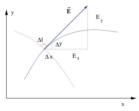
Figure 7.1: The electric field is tangent at each point of an electric field line and perpendicular to an equipotential line. By approximating the continuous curve by the line segment  $\Delta l$ , we have that  $\Delta y/\Delta x = E_y/E_x$ .
