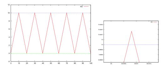
Figure 2.20: The trajectory x(t) of a particle in a box with L = 10,  $x_0 = 0.0$ ,  $v_0 = 1.0$ ,  $t_0 = 0$ ,  $\delta t = 0.01$ . The plot to the right magnifies a detail when  $t \approx 90$  which exposes the systematic errors in determining the exact moment of the collision of the particle with the wall at  $t_k = 90$  and the corresponding maximum value of x(t),  $x_m = L = 10.0$ .
