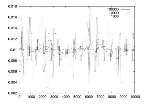
Figure 11.5: The relative frequency distribution of the pseudorandom numbers generated by drandom() as a function of the sample size n for n = 1000, 10000, 100000.
