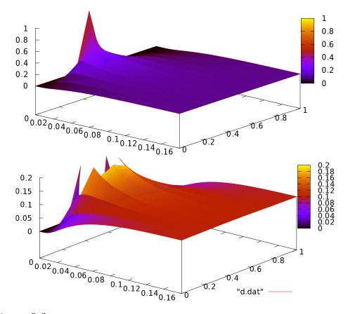
Figure 8.6: The function u(x,t) for  $N_x = 10$ ,  $N_t = 100$ ,  $t_f = 0.16$ . The second plot differs only in the scale of the *z* axis so that we can easily see the details of the diffusion away from the point  $x_0 \equiv x_{N_x/2} = x_5$ .
