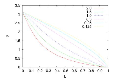
Figure 5.13: The impact parameter  $b(\theta)$  for the potential given by equation (5.27) for different values of the initial velocity v. We set a = 1, x(0) = -5 and made 4000 integration steps from  $t_i = 0$  to  $t_f = 40$ .
