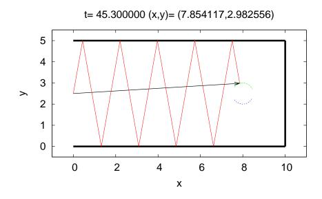
Figure 2.24: The trajectory of the particle calculated by the program MiniGolf.f90 using the parameters chosen in the text. The moment of ... success is shown. At time t = 45.3 the particle enters the hole's region which has its center at (8, 2.5) and its radius is 0.5.
