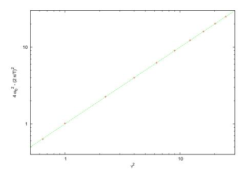
Figure 4.22: The period of oscillation of the damped oscillator for several values of  $\gamma$  and  $\omega_0 = 3.145$ . The axes are chosen so that equation (4.28)  $(2\pi/T)^2 = 4\omega_0^2 - \gamma^2$  can be easily verified. The points in the plot are our measurements whereas the straight line is the theoretical prediction, the diagonal y = x
