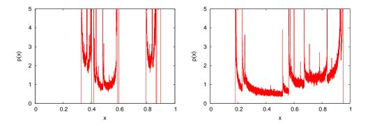
Figure 3.10: The distribution functions p(x) of x of the logistic map for r = 3.59 (left) and 3.8 (right). The chaotic behavior appears to be weaker for r = 3.59, and this is reflected on the value of the entropy. One sees that there exist intervals of x with p(x) = 0 which become smaller and vanish as r gets close to 4. This distribution is very hard to be distinguished from a truly random distribution.
