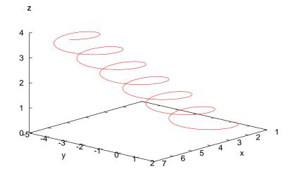
Figure 6.2: The trajectory of a charged particle in a constant magnetic field  $\vec{B} = B\hat{z}$ , where qB/m = 1.0 and a constant electric field  $\vec{E} = E_x \hat{x} + E_y \hat{y} \ \mu \epsilon \ qE_x/m = qE_y/m = 0.1$ .  $\vec{v}(0) = 1.0\hat{y} + 0.1\hat{z}$ ,  $\vec{r}(0) = 1.0\hat{x}$ . The integration of the equations of motion is performed using the RK45 method from  $t_0 = 0$  to  $t_f = 40$  with 1000 steps. Each axis is on a different scale.
