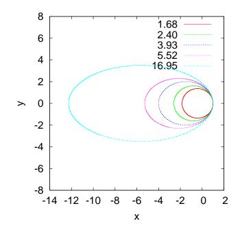
Figure 5.5: Planetary trajectories for GM = 10, x(0) = 1.0, y(0) = 0,  $v_{0y} = 0$  and  $v_{0x} = 3.6$ , 3.8, 4.0, 4.1, 4.3. The numbers are the corresponding half periods.
