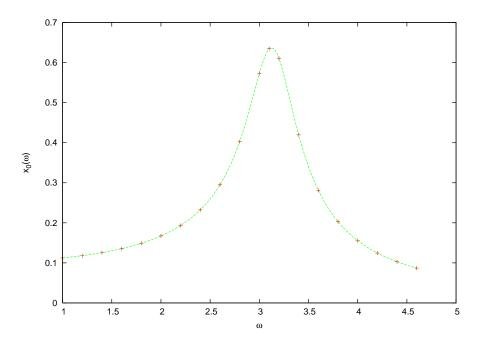
Figure 4.24: The oscillation amplitude  $x_0(\omega)$  as a function of  $\omega$  for the forced damped oscillator, where  $\omega_0 = 3.145$ ,  $\gamma = 0.5$  and  $a_0 = 1.0$ . We observe a resonance for  $\omega \approx \omega_0$ . The points of the plot are our measurements and the line is the theoretical prediction given by equation (4.33).
