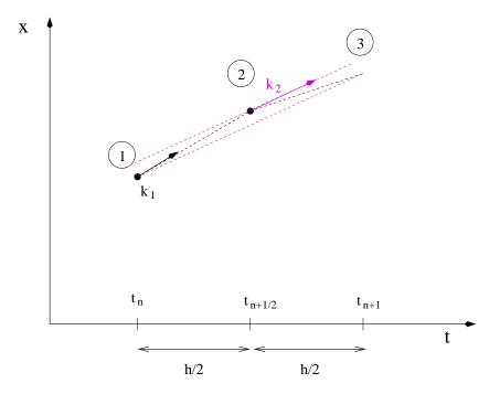
Figure 4.9: The geometry of an integration step of the 2nd order Runge-Kutta method given by equation (4.19).
