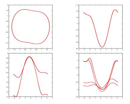
Figure 4.27: A phase space trajectory of the forced damped pendulum. The parameters chosen are  $\omega_0 = 1.0$ ,  $\omega = 2.0$ ,  $\gamma = 0.2$  and A = 0.60, 0.72, 0.85, 1.02. We observe the phenomenon of period doubling.
