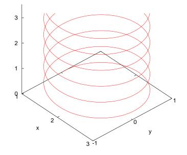
Figure 6.1: The trajectory of a charged particle in a constant magnetic field  $\vec{B} = B\hat{z}$ , where qB/m = 1.0,  $\vec{v}(0) = 1.0\hat{y} + 0.1\hat{z}$ ,  $\vec{r}(0) = 1.0\hat{x}$ . The integration of the equations of motion is performed using the RK45 method from  $t_0 = 0$  to  $t_f = 40$  with 1000 steps.
