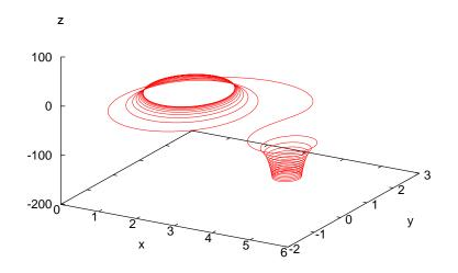
Figure 6.3: The trajectory of a charged particle in a magnetic field  $\vec{B} = B_y \hat{y} + B_z \hat{z}$ with  $qB_y/m = -0.02y$ ,  $qB_z/m = 1 + 0.02z$ ,  $\vec{v}(0) = 1.0\hat{y} + 0.1\hat{z}$ ,  $\vec{r}(0) = 1.0\hat{x}$ . The integration of the equations of motion is performed using the RK45 method from  $t_0 = 0$ to  $t_f = 500$  with 10000 steps. Each axis is on a different scale.
