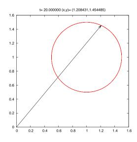
Figure 2.5: The particle trajectory plotted by the gnuplot program in the file animate2D.gnu of the accompanied software. The position vector is shown at a given time t, which is marked on the title of the plot together with the coordinates (x,y). The data is produced by the program Circle.f90 described in the text.
