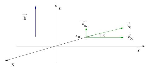
Figure 2.16: A particle at time  $t_0 = 0$  is at the position  $\vec{r}_0 = x_0 \hat{x}$  with velocity  $\vec{v}_0 = v_{0y}\hat{y} + v_{0z}\hat{z}$  in a homogeneous magnetic field  $\vec{B} = B\hat{z}$ .
