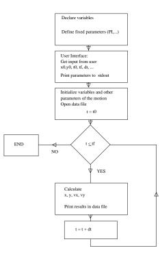
Figure 2.2: The flowchart of a typical program computing the trajectory of a particle from its (kinematic) equations of motion.
