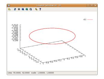
Figure 2.14: The plot of the particle trajectory  $\vec{r}(t)$  of the program ConicalPendulum.f90 for  $\omega = 6.28$ , l = 1.0. We can click and drag with the mouse on the window and rotate the curve and see it from a different angle. At the bottom left of the window, we see the viewing direction, given by the angles  $\theta = 55.0$  degrees (angle with the *z* axis) and  $\phi = 62$  degrees (angle with the *x* axis).
