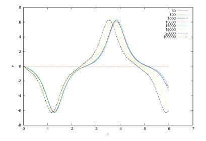
Figure 4.7: Convergence of the Euler-Verlet method, similarly to figure 4.5. We observe a faster convergence compared to Euler's method but that the roundoff errors make the results unstable for  $Nt \gtrsim 18,000$ .
