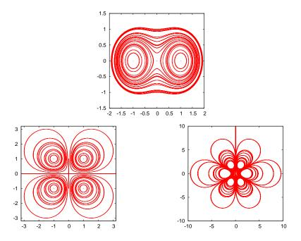
Figure 7.5: Equipotential lines of the electric field generated by a point charge distribution on the plane calculated by the program in EPotential.f90. Beware: the density of the lines is not correctly calculated and it is not proportional to the magnitude of the electric field. See problem 7.5.
