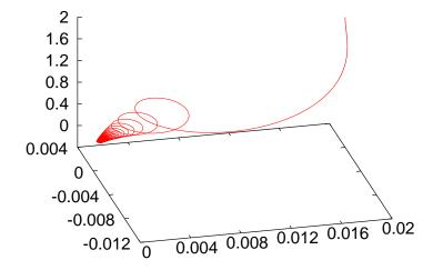
Figure 6.8: The trajectory of a charged particle in a magnetic dipole field given by equation (6.11). We used  $B_0 = 1000$ ,  $\vec{r} = 0.02\hat{x} + 2.00\hat{z}$ ,  $\vec{v} = -0.99999\hat{z}$ . The integration was done from  $t_0 = 0$  to  $t_f = 5$  in 10000 steps.
