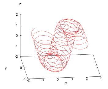
Figure 6.4: The trajectory of a charged particle in a magnetic field  $\vec{B} = B_y \hat{y} + B_z \hat{z}$  with  $qB_y/m = 0.08z$ ,  $qB_z/m = 1.4 + 0.08y$ ,  $\vec{v}(0) = 1.0\hat{y} + 0.1\hat{z}$ ,  $\vec{r}(0) = 1.0\hat{x}$ . The integration of the equations of motion is performed using the RK45 method from  $t_0 = 0$  to  $t_f = 3000$  with 40000 steps. Each axis is on a different scale.
