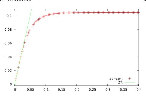
Figure 8.5: The expectation value  $\langle r^2 \rangle_j$  as a function of  $t_j$  for  $N_x = 10$ ,  $N_t = 100$ ,  $t_f = 0.4$ . For small values of  $t_j$  we obtain  $\langle r^2 \rangle_j \approx 2t_j$ . The solid line is the straight line 2t.
