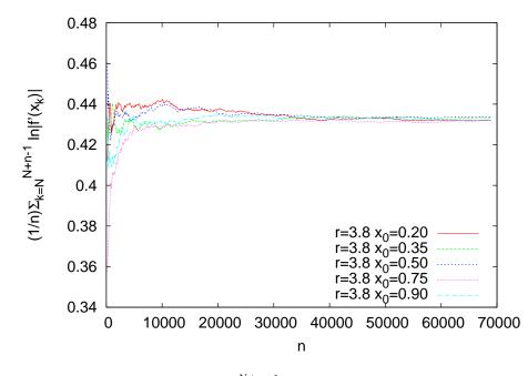
Figure 3.8: Plot of the sum  $(1/n) \sum_{k=N}^{N+n-1} \ln |f'(x_k)|$  as a function of *n* for the logistic map with r = 3.8, N = 2000 for different initial conditions  $x_0 = 0.20, 0.35, 0.50, 0.75, 0.90$ . The different curves converge in the limit  $n \to \infty$  to  $\lambda = 0.4325(10)$ .
