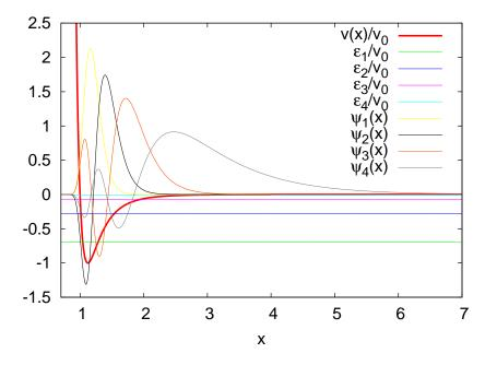
Figure 10.9: The four bound states for the Lennard-Jones potential with  $v_0 = 250$ . The bold red line is the potential  $v(x)/v_0$ . We plot the energy levels  $\epsilon_n/v_0$  and the corresponding wave functions.
