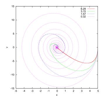
Figure 4.20: The phase space trajectory for the damped oscillator for several values of  $\gamma$  and  $\omega_0 = 3.145$ . Note the attractor at (x, v) = (0, 0) where all trajectories are "attracted to" as  $t \to +\infty$ .
