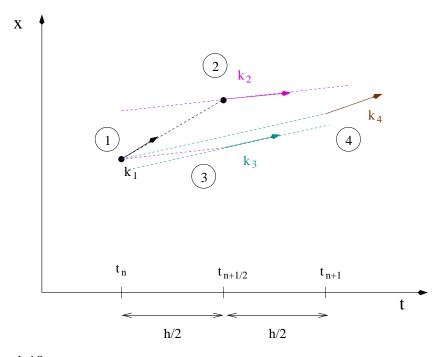
Figure 4.10: The geometry of an integration step of the Runge-Kutta method of 4th order given by equation (4.20).
