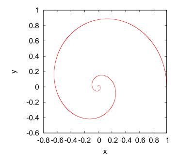
Figure 5.7: The spiral orbit of a particle moving under the influence of a central force  $\vec{F} = -k/r^3\hat{r}$ .
