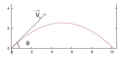
Figure 2.7: The trajectory of a particle moving under the influence of a constant gravitational field. The initial conditions are set to x(0) = y(0) = 0,  $v_x(0) = v_{0x} = v_0 \cos \theta$  and  $v_y(0) = v_{0y} = v_0 \sin \theta$ .
