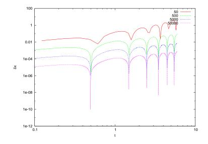
Figure 4.11: The discrepancy of the numerical results of the Euler method from the analytic solution for the simple harmonic oscillator. The parameters chosen are  $\omega^2 = 10$ ,  $t_i = 0, t_f = 6, x(0) = 0.2, v(0) = 0$  and the number of steps is N = 50, 500, 5, 000, 50, 000. Observe that the error becomes approximately ten times smaller each time according to the expectation of being of order  $\sim O(\Delta t)$ .
