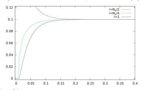
Figure 8.4: The functions  $u_{N_x/2,j}$ ,  $u_{N_x/4,j}$ ,  $u_{1,j}$  are given as a function of  $t_j$  for  $N_x = 10$ ,  $N_t = 100$ ,  $t_f = 0.4$ . We observe that for large times they are consistent with uniform diffusion.
