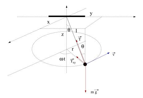
Figure 2.12: The conical pendulum of the program ConicalPendulum.f90.
