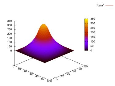
Figure 7.9: The solution of equation (7.13) by the program in the file Poisson.f90 for L= 51, V= 0 on the boundary and the charge  $4\pi Q = 1000$  uniformly distributed in a small square with sides made of 10 lattice sites.
