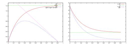
Figure 2.9: The plots of x(t),y(t) (left) and  $v_x(t),v_y(t)$  (right) from the data produced by the program ProjectileAirResistance.f90 for k = 5.0,  $v_0 = 10.0$ ,  $\theta = \pi/4$ ,  $t_f = 0.91$  and  $\delta t = 0.001$ . We also plot the asymptotes of these functions as  $t \to \infty$ .
