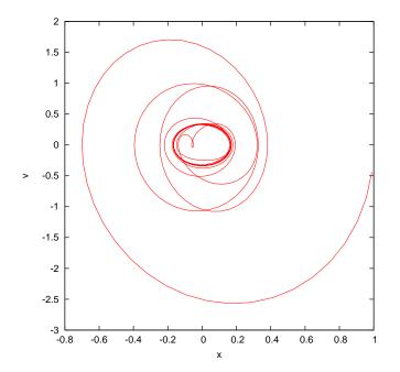
Figure 4.25: A phase space trajectory of the forced damped oscillator with  $\omega_0 = 3.145$ ,  $\omega = 2.0$ ,  $\gamma = 0.5$  and  $a_0 = 1.0$ . The harmonic oscillation which is the steady state of the system is an ellipse, which is an attractor of all the phase space trajectories that correspond to different initial conditions.
