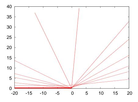
Figure 5.10: Rutherford scattering trajectories. We set  $k_1 \equiv \frac{qQ}{4\pi\epsilon_0 m} = 1$  (see code in the file rk2\_cb.f90) and b = 0.08, 0.015, 0.020, 0.035, 0.080, 0.120, 0.200, 0.240, 0.320, 0.450, 0.600, 1.500. The initial position of the particle is at x(0) = -50 and its initial velocity is v = 3 in the *x* direction. The number of integration steps is 1000, the initial time is 0 and the final time is 30.
