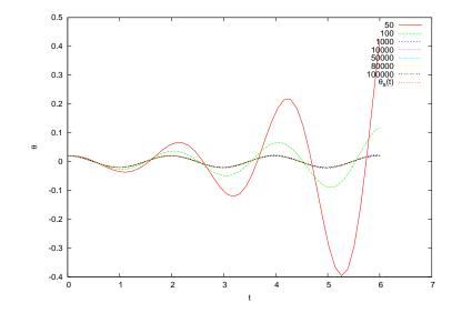
Figure 4.2: Convergence of Euler's method for a simple pendulum with period  $T \approx 1.987(\omega^2 = 10.0)$  for several values of the time step  $\Delta t$  which is determined by the number of integration steps Nt= 50-100,000. The solution is given for  $\theta_0 = 0.2$ ,  $\omega_0 = 0.0$  and we compare it with the known solution for small angles with  $\alpha(t) \approx -(g/l) \theta$ .
