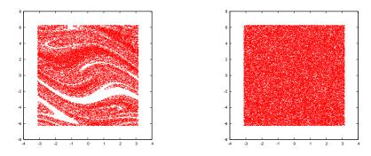
Figure 4.31: Basin of attraction for the forced damped pendulum. The parameters chosen are  $\omega_0 = 1.0$ ,  $\omega = 2.0$ ,  $\gamma = 0.2$  and A = 0.85, 1.4.
