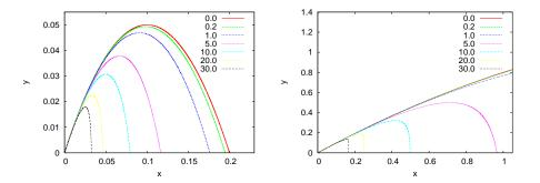
Figure 5.3: The trajectory of a projectile moving in a constant gravitational field  $\vec{g} = -10 \hat{y}$  with air resistance causing acceleration  $\vec{a}_r = -k\vec{v}$  for k = 0, 0.2, 1, 5, 10, 20, 30. The left plot has  $\vec{v}(0) = \hat{x} + \hat{y}$  and the right plot has  $\vec{v}(0) = 5\hat{x} + 5\hat{y}$ .
