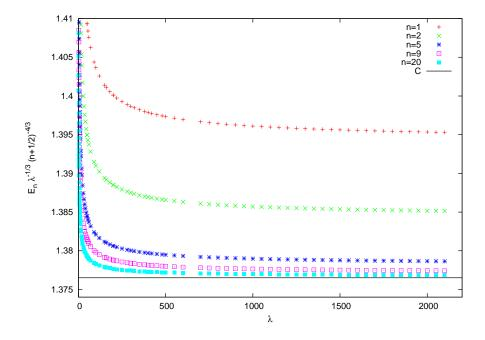
Figure 9.6: Test of the asymptotic relation (9.32). The vertical axis is  $E_n \lambda^{-1/3} (n + 1/2)^{-4/3}$  where for large enough n and  $\lambda$  should approach the value  $C = 3^{4/3} \pi^2 / \Gamma(1/4)^{8/3} \approx 1.37650740$  (horizontal line).
