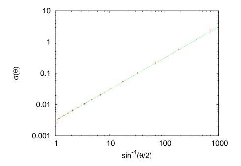
Figure 5.12: Differential cross section of the Rutherford scattering like in figure 5.11. The solid line is the function  $1/(4 \times 3^4)x$  from which we can deduce the functional form of  $\sigma(\theta)$ .
