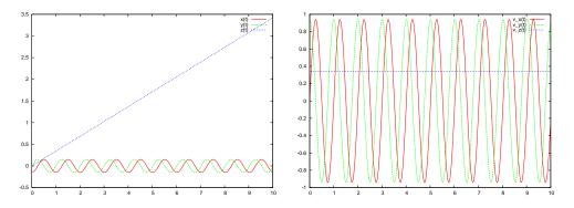
Figure 2.17: The plots of the  $x(t), y(t), z(t), v_x(t), v_y(t), v_z(t)$  functions calculated by the program in ChargeInB.f90 for  $\omega = 6.28$ ,  $x_0 = 1.0$ ,  $\theta = 20$  degrees.
