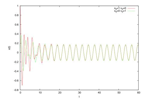
Figure 4.23: The period of oscillation for the forced damped oscillator for different initial conditions. We have chosen  $\omega_0 = 3.145$ ,  $\omega = 2.0$ ,  $\gamma = 0.5$  and  $a_0 = 1.0$ . We note that after the transient behavior the system oscillates harmonically according to the relation  $x(t) = x_0(\omega) \cos(\omega t + \delta)$ .
