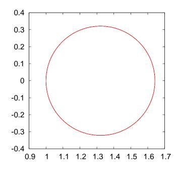
Figure 6.6: Projection of the trajectory of a relativistic charged particle in a magnetic field  $\vec{B} = B_z \hat{z}$  with  $qB_z/m_0 = 10.0$ , on the *xy* plane.  $\vec{v}(0) = 0.95\hat{y} + 0.10\hat{z}$ ,  $\vec{r}(0) = 1.0\hat{x}$ . The integration is performed by using the RK45 method from  $t_0 = 0$  to  $t_f = 20$  with 1000 steps. Each axis is on a different scale.
