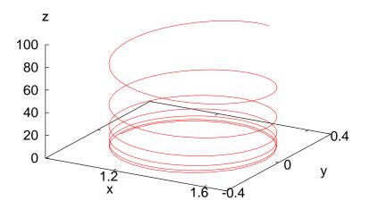
Figure 6.7: The influence of an additional electric field  $q\vec{E}/m_0 = 1.0\hat{z}$  on the trajectory shown in figure 6.5.
