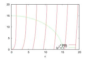
Figure 3.6: Plots of the right and left hand sides of equation (3.24). The intersections of the curves determine the solutions of the equation and their approximate graphical estimation can serve as initial points  $x_0$  for the Newton-Raphson method.
