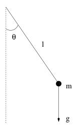
Figure 4.1: A simple pendulum of length *l* in a homogeneous gravitational field *g*.
