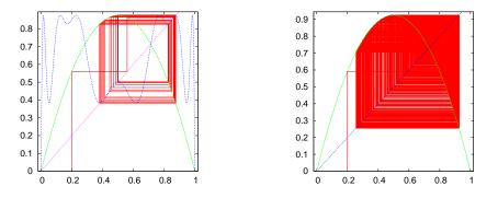
Figure 3.3: (Left) A 4-cycle for r = 3.5. The blue curve is  $y = f^{(4)}(x)$  which intersects the diagonal at four points determined by  $x_{\alpha}$ ,  $\alpha = 5, 6, 7, 8$ . The four cycle passes through these points. (Right) a non periodic orbit for r = 3.7 when the system exhibits chaotic behavior.
