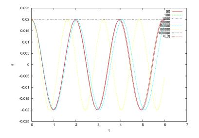
Figure 4.4: Convergence of the Euler-Verlet method, similarly to figure 4.2. We observe a faster convergence than Euler's method, but the roundoff errors make the results useless for  $Nt \gtrsim 50,000$  (note what happens when Nt = 100,000. Why?).
