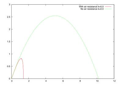
Figure 2.10: Trajectories of the particles shot with  $v_0 = 10.0$ ,  $\theta = \pi/4$  in the absence of air resistance and when the air resistance is present in the form  $\vec{F} = -mk\vec{v}$  with k = 5.0.
