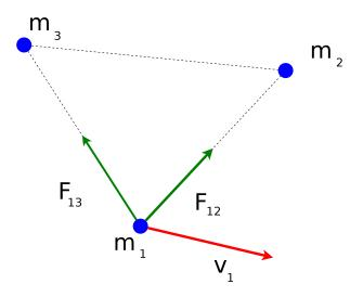
Figure 5.17: Three particles of equal mass interact via their mutual gravitational attraction. The problem is solved numerically using the program in the files rkA.f90, rkA\_3pcb.f90. The same program can be used in order to study the motion of three equal charges under the influence of their attractive or repulsive electrostatic force.
