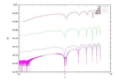
Figure 4.14: Like in figure 4.11 for the 4th order Runge–Kutta method. The error becomes approximately  $10^{-4}$  times smaller each time according to the expectation of being of order ~  $\mathcal{O}(\Delta t^4)$ . The roundoff errors become apparent for 50,000 steps.
