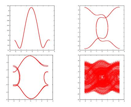
Figure 4.29: A phase space trajectory of the forced damped pendulum. The parameters chosen are  $\omega_0 = 1.0$ ,  $\omega = 2.0$ ,  $\gamma = 0.2$  and A = 1.568, 3.8, 4.44, 4.5. We observe the system exiting and reentering regimes of chaotic behavior.
