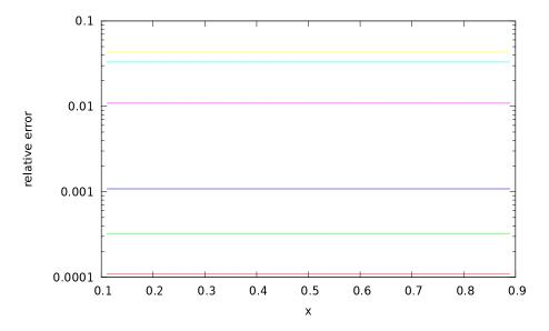
Figure 8.3: The absolute value of the relative error of the numerical computation for Nx=10, Nt=800, tf= 2 for different times  $t_j$ . We take j = 3, 7, 21, 201, 601, 781 and observe that the relative error increases with j.
