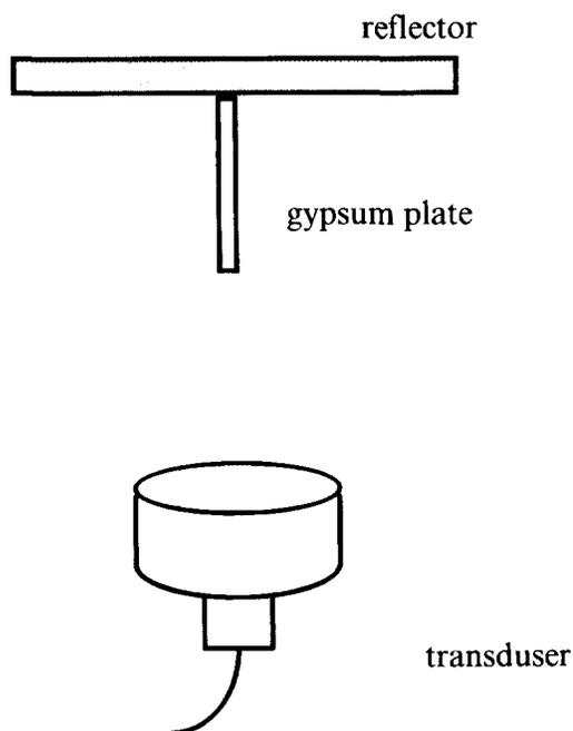
Fig. 3. Erosion under standing wave.
