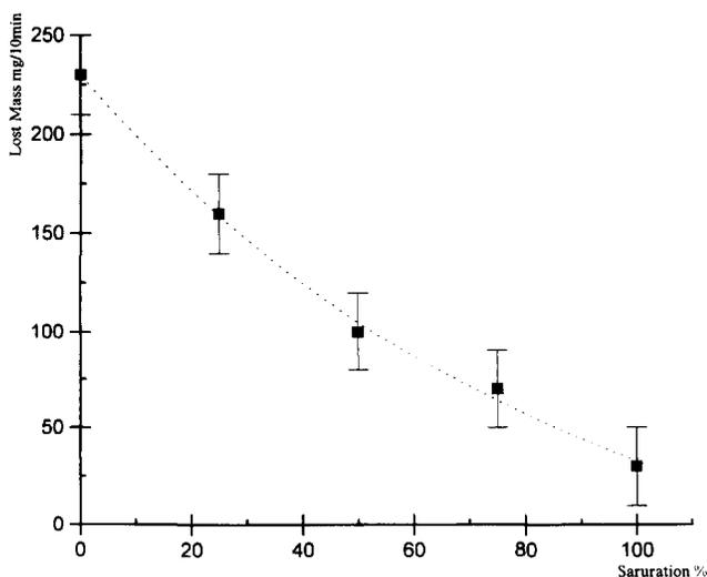
Fig. 2. Mass of gypsum plates lost by ultrasonic erosion as a function of solution saturation.
