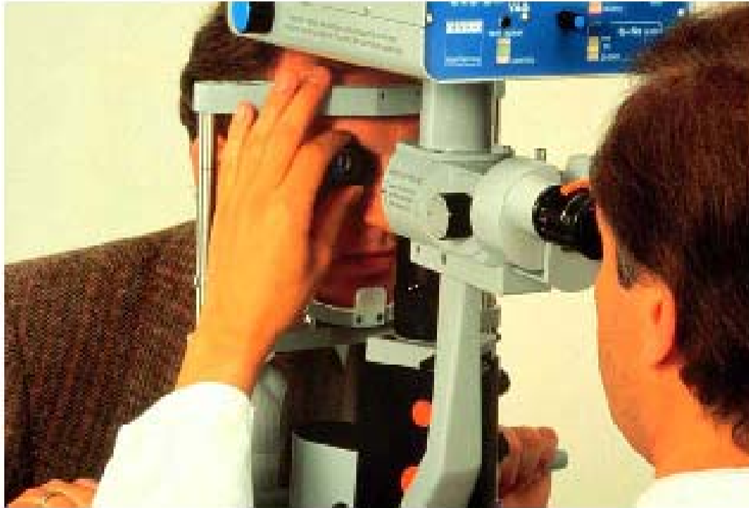
Fig. 12. Q-switched Nd:YAG laser attached to an ophthalmologic slit lamp (Photo: Carl Zeiss).
