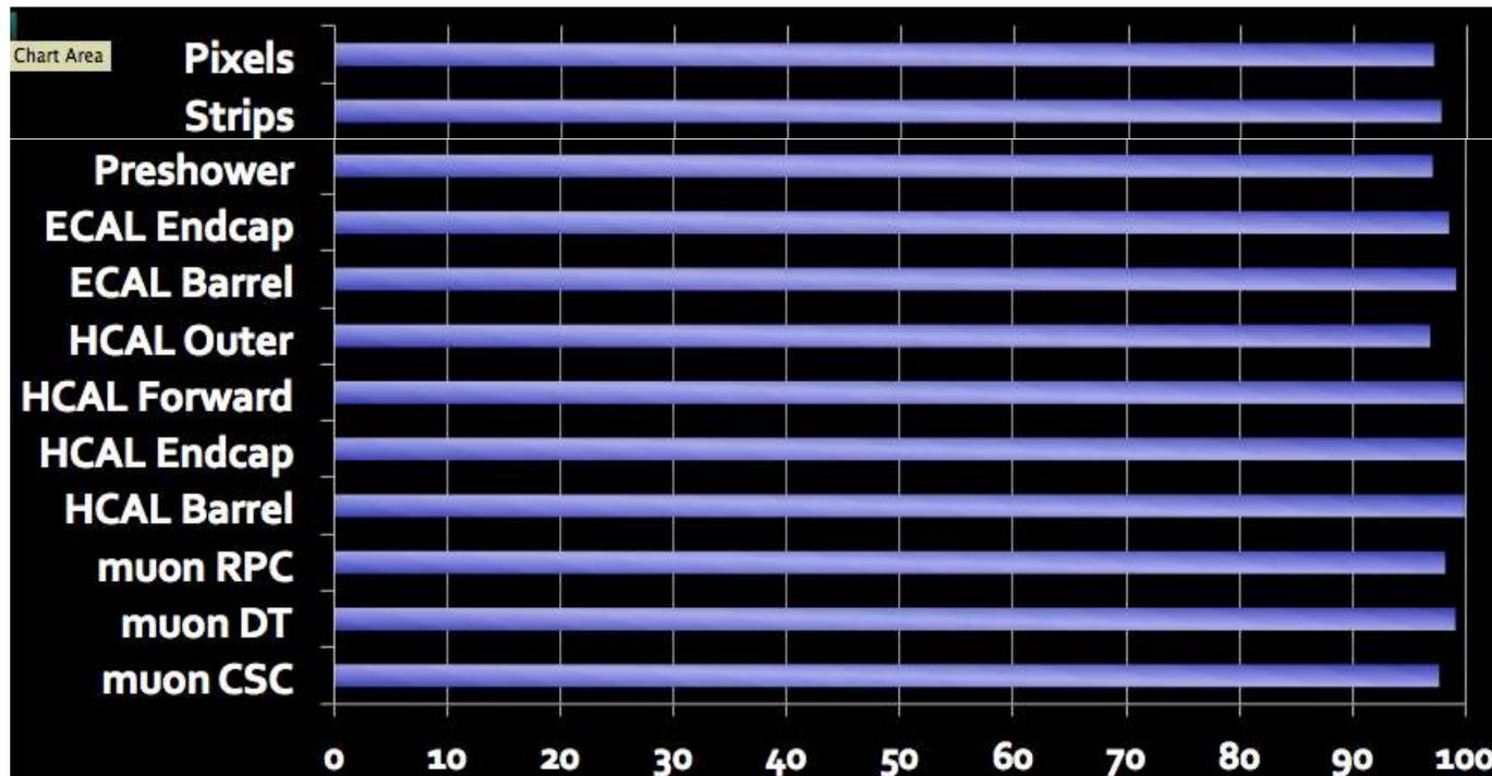
The fraction of working channels is >98%
