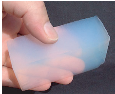
FIGURE 44 A piece of aerogel, a solid that is so porous that it is translucent (courtesy NASA).
