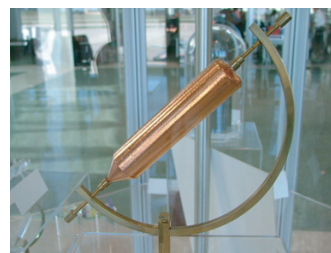
FIGURE 38 Synthetic copper single crystal, picture width 30 cm (© Lachlan Cranswick).
