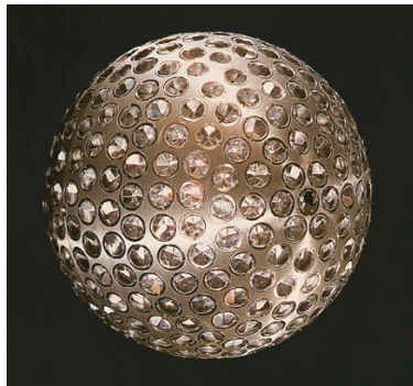
FIGURE 65 The LAGEOS satellites: metal spheres with a diameter of 60 cm, a mass of 407 kg, and covered with 426 retroreflectors (NASA).
