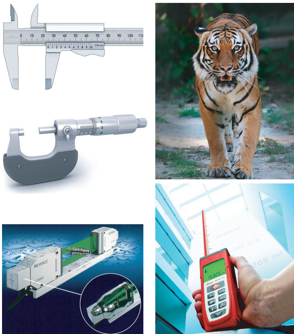
FIGURE 23 Three mechanical (a vernier caliper, a micrometer screw, a moustache) and three optical (the eyes, a laser meter, a light curtain) length and distance measurement devices (© www.medien-werkstatt.de , Naples zoo, Leica Geosystems and Keyence).
