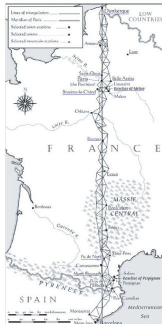
FIGURE 107 The measurements that lead to the definition of the metre (© Ken Alder).
