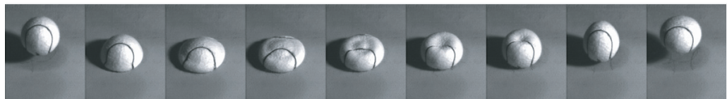
FIGURE 6 An example of how precision of observation can lead to the discovery of new effects: the deformation of a tennis ball during the c. 6 ms of a fast bounce (© International Tennis Federation).
