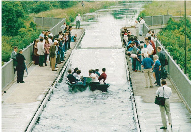
FIGURE 170 A solitary water wave followed by a motor boat, reconstructing the discovery by Scott Russel (© Dugald Duncan).
