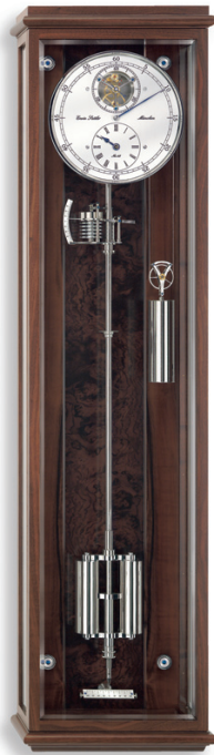
FIGURE 106 A precision second pendulum, thus about 1 m in length; almost at the upper end, the vacuum chamber that compensates for changes in atmospheric pressure; towards the lower end, the wide construction that compensates for temperature variations of pendulum length; at the very bottom, the screw that compensates for local variations of the gravitational acceleration, giving a final precision of about 1 s per month (© Erwin Sattler OHG).
