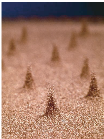
FIGURE 215 Oscillons formed by shaken bronze balls; horizontal size is about 2 cm (© Paul Umbanhowar)
