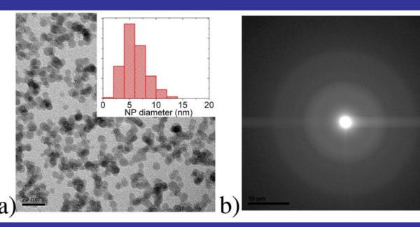
> TEM images showing the amorphous  $TiO_2$  nps used in the memristor
