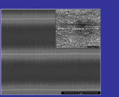
Silver nanoparticles selfassembled into nanowires
