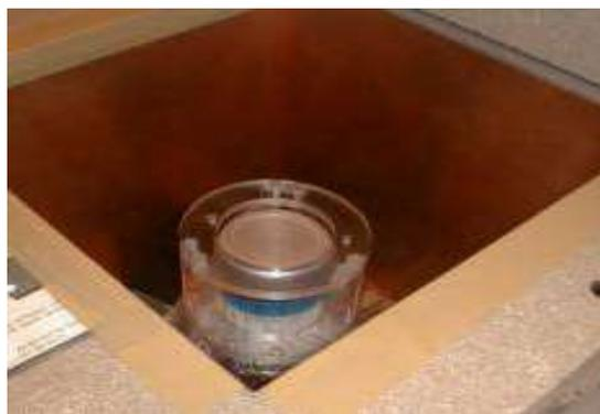
**Figure 2.8:** High Purity Germanium detector (HPGe) at NED-NTUA
