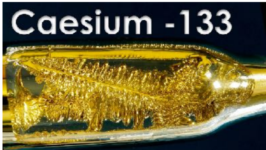
1 second = time duration of 9.192.631.770 periods of the radiation corresponding to the transition between the two hyperfine levels of the ground state of the caesium-133 atom.
