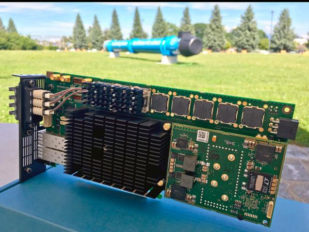
common readout unit (world's largest FPGA)
