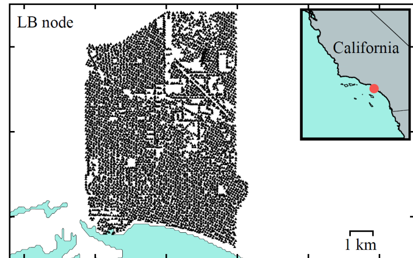
An array of 5200 nodes installed in Long Beach, California. Note the 1 km scale. (From Li, 2021)
