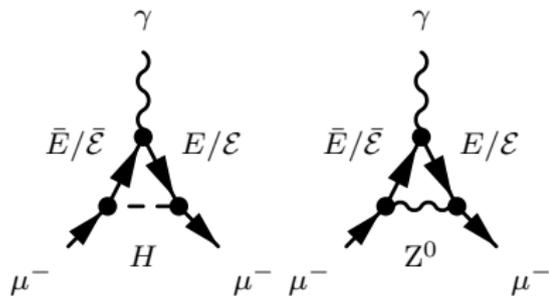
Non-zero mixings with VLLs induce **lepton flavour violating** (LFV) vertices are **generated** (mainly involving  $\mu$  decays)  $\rightarrow$  Model implemented in SARAH, Sphenox and flavio to compute LFV observables.
