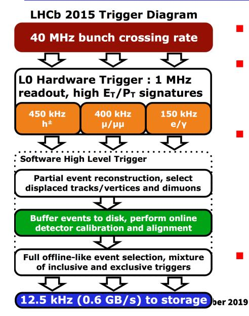
After LHCb's hardware trigger, events are buffered.
