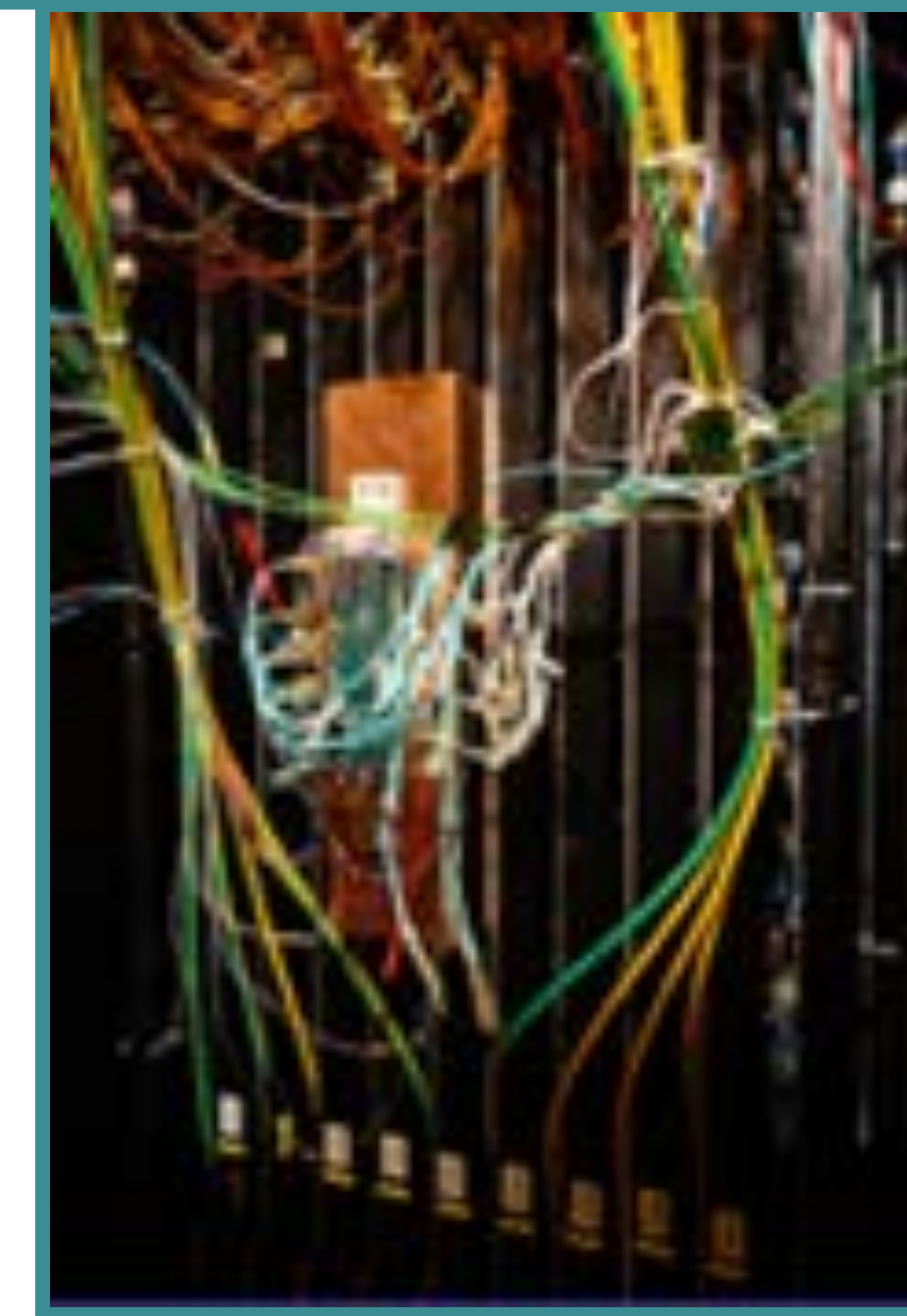
RICH MaPMTs under test
