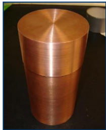
Housing made at LSC of electroformed copper
