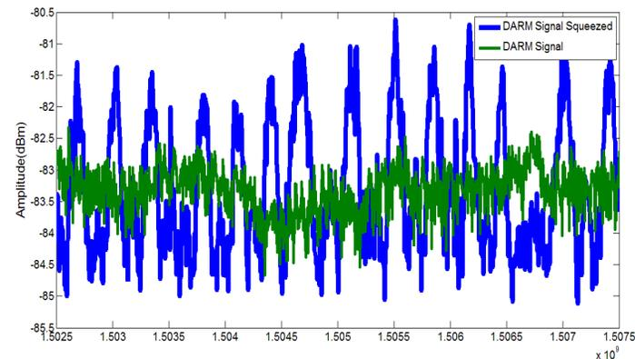
Figure: The blue curve represents the output of the DARM signal when the squeezed light was injected into the interferometer and the green one is the Shot Noise Limit of the DARM output. There is around 2dB of Squeezing at 5MHz.
