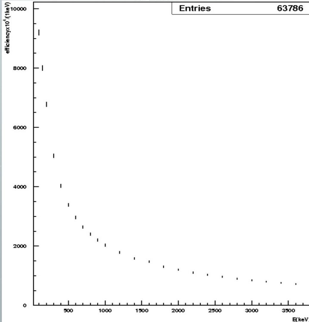
Simulated detection efficiency for  $\gamma$ s produced inside the Germanium detector, multiplied by  $10^4$
