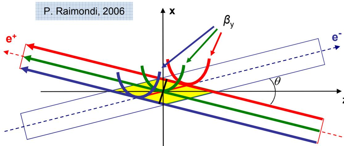
$$\phi = \frac{\sigma_z}{\sigma_x} \operatorname{tg}\left(\frac{\theta}{2}\right) - \text{Piwinski angle, should be } \gg 1$$
