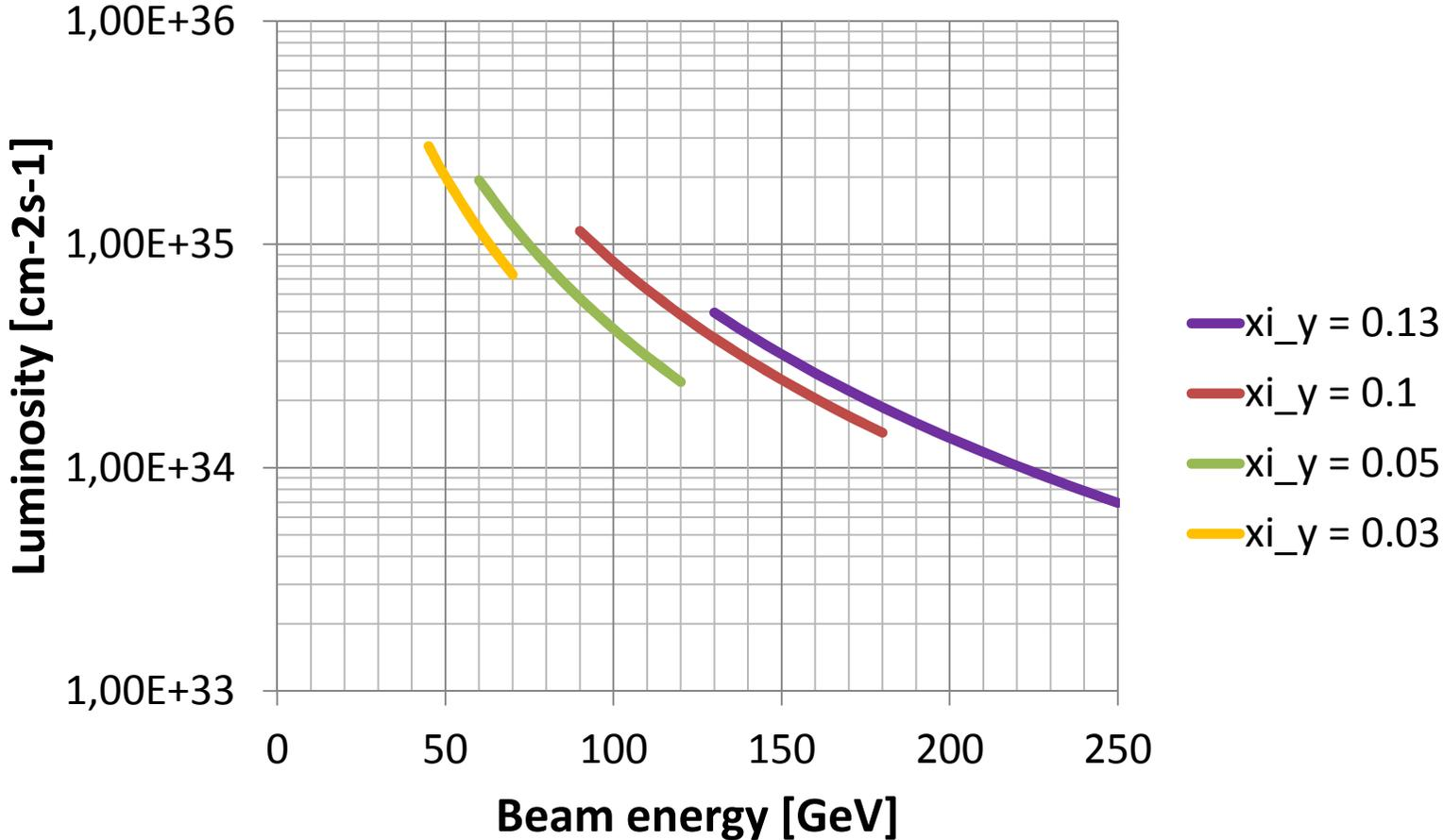
Luminosity for an 11km radius machine, with 50MW power consumption,  $\beta^*_y$  of 1mm (and longitudinal beam size of 1.2mm)
