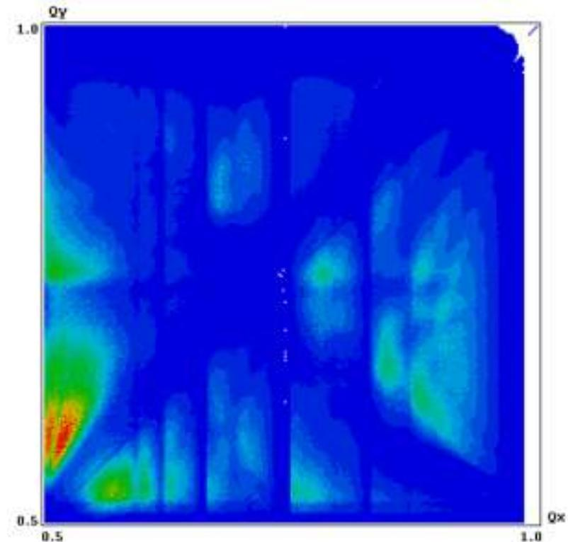
Tune scan for FCC-ee head-on collision scheme without CW (120 GeV)
