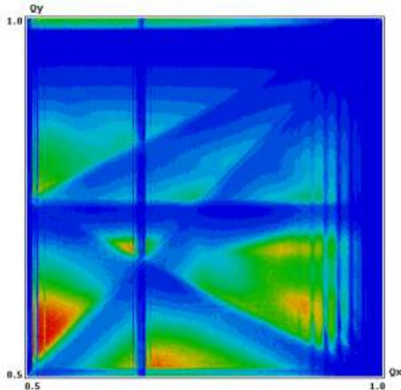
Typical tune scan for CW scheme with high beam-beam parameter ( $\sim 0.2$ ) for a Super  $c\text{-}\tau$  factory
