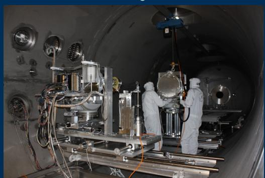
Preparation of PANTER X-ray Tests (FM-3c)
