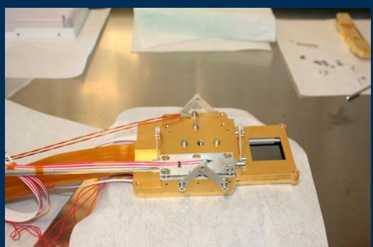
Cold part of Camera (with test sensors)
