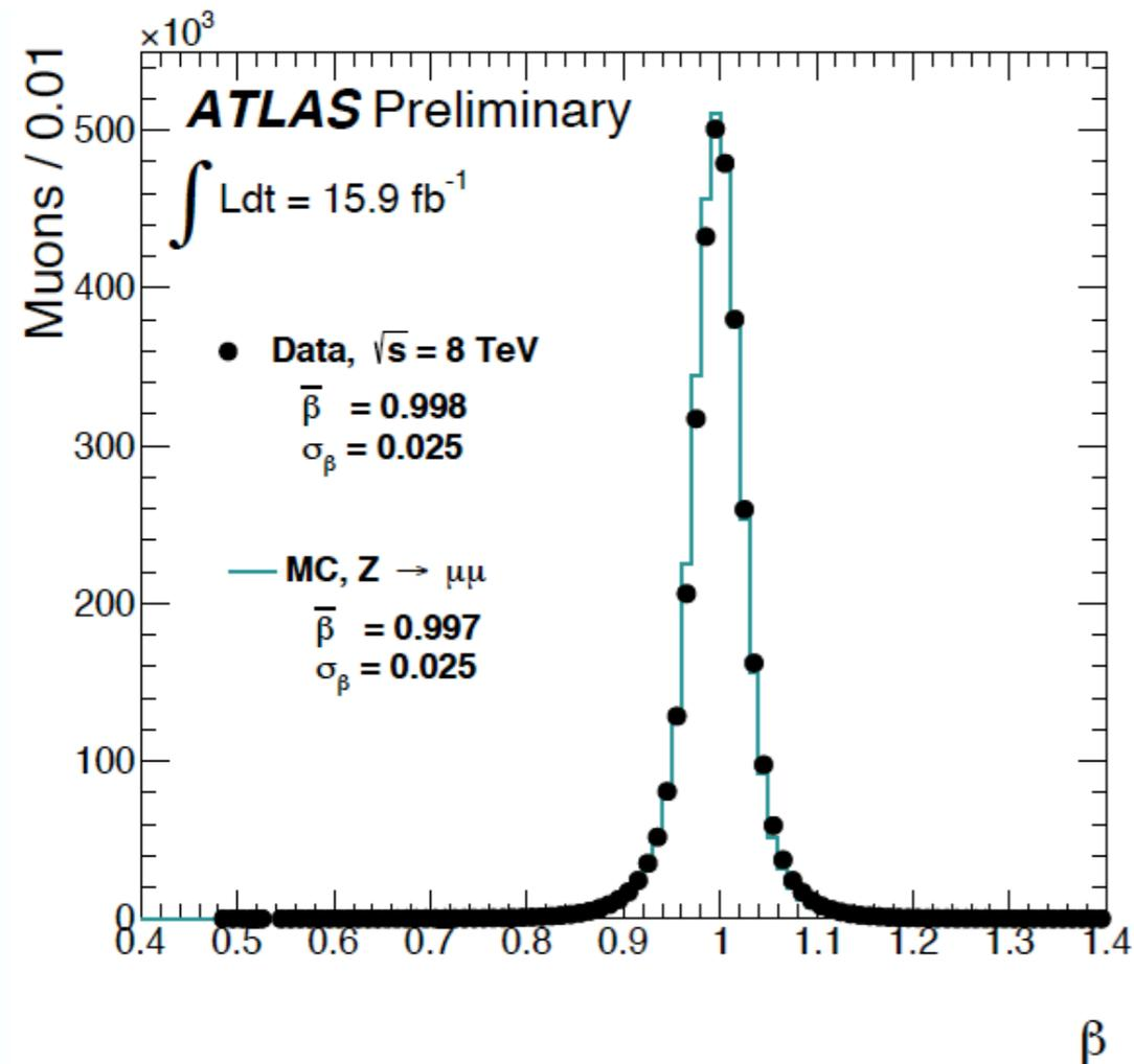
Distribution of the combined measurement for selected muons in data and  $Z \rightarrow \mu\mu$  decays in MC simulation. The typical resolutions are 0.025.
