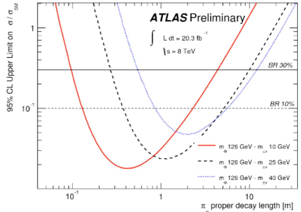
Observed 95% CL limits on  $\sigma \times \text{BR}$  for a light Higgs boson with 125 GeV mass and three different  $\pi_\nu$  masses as a function of the  $\pi_\nu$  proper decay length
