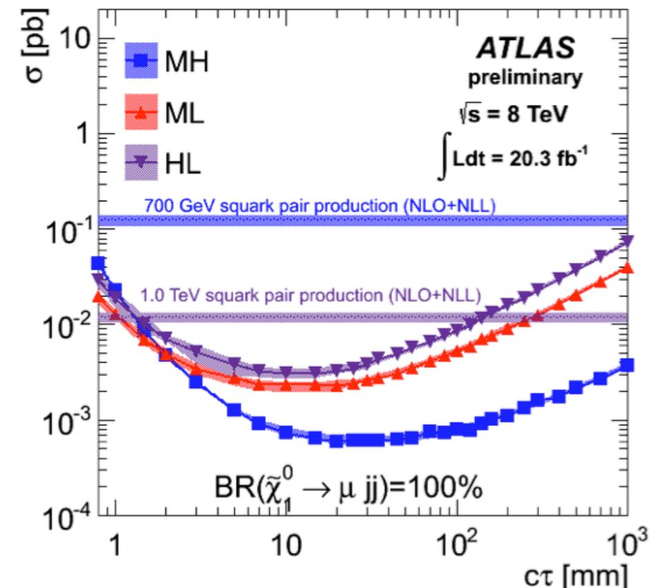
Upper limits at 95% CL on  $\sigma$  vs the neutralino lifetime for different combinations of squark and neutralino masses
