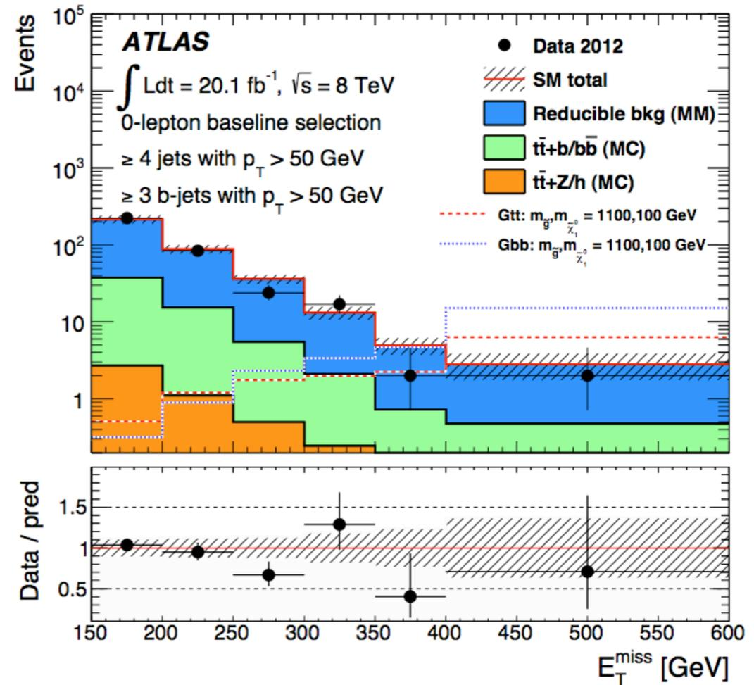
The observed distributions of  $m_{\text{eff}}^{4j}$  and  $E_{\text{T}}^{\text{miss}}$  after the 0-lepton baseline selection, together with the background prediction. Also displayed are the respective contributions of the backgrounds described in the legend and the ratio between the expected and observed event yields.
