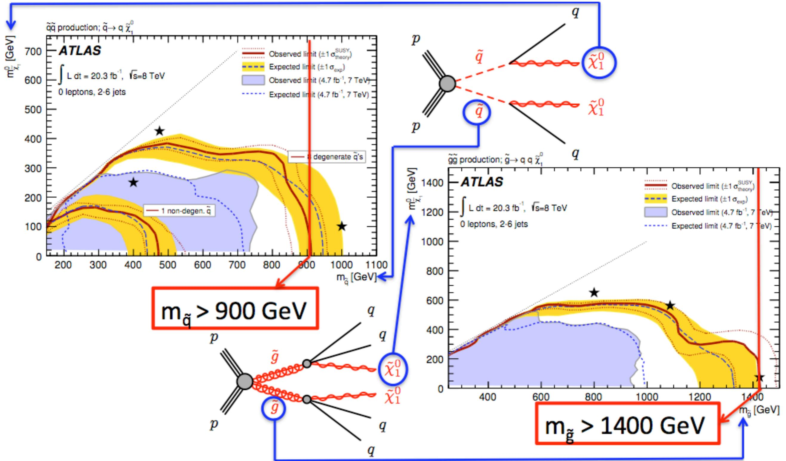
Exclusion limits for direct production of light-flavor squark pairs and of gluino pairs. Gluinos (light-flavor squarks) are required to decay to two quarks (one quark) and a neutralino LSP.
