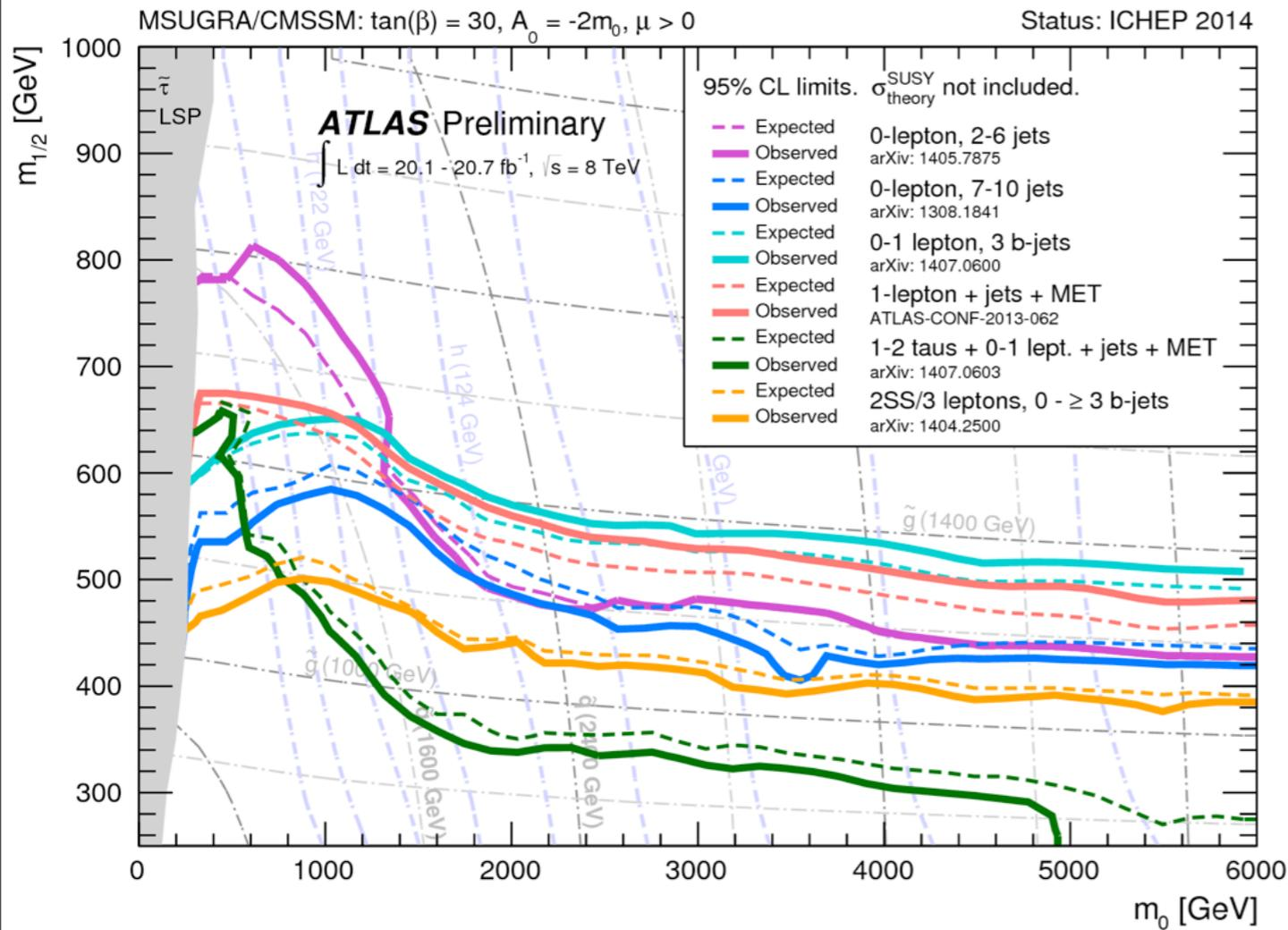
**Exclusion limits at 95% CL for 8 TeV analyses in the  $(m_0, m_{1/2})$  plane for the MSUGRA/CMSSM model with the remaining parameters set to  $\tan(\beta) = 30, A_0 = -2m_0, \mu > 0$ . Part of the model plane accommodates a lightest neutral scalar Higgs boson mass of 125 GeV**
