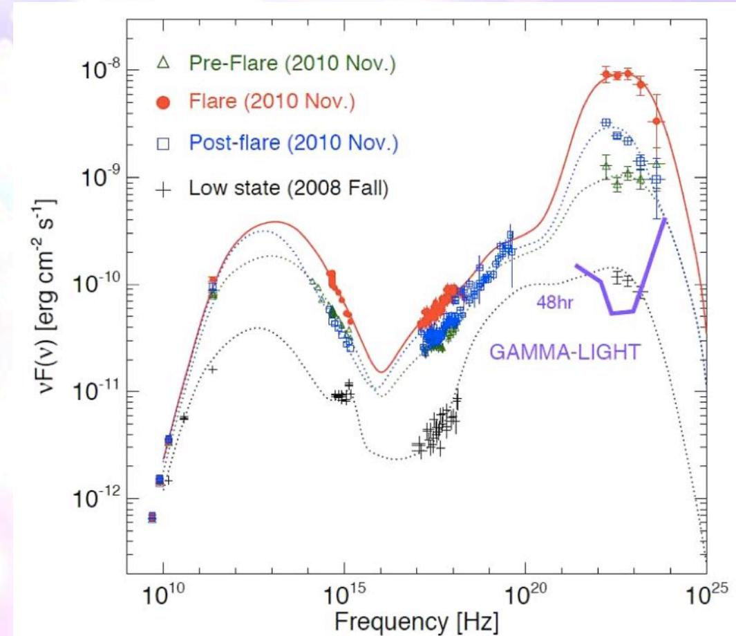
G-LIGHT will allow us to investigate daily (or sub-daily) SEDs during gamma-ray super-flares. The 5-sigma G-LIGHT differential sensitivity (purple line) is computed for an integration time of 48 hours
