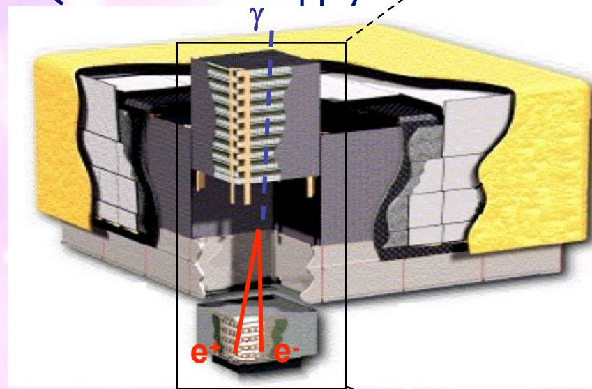
An anticoincidence detector around the telescope distinguishes gamma-rays from charged particles
