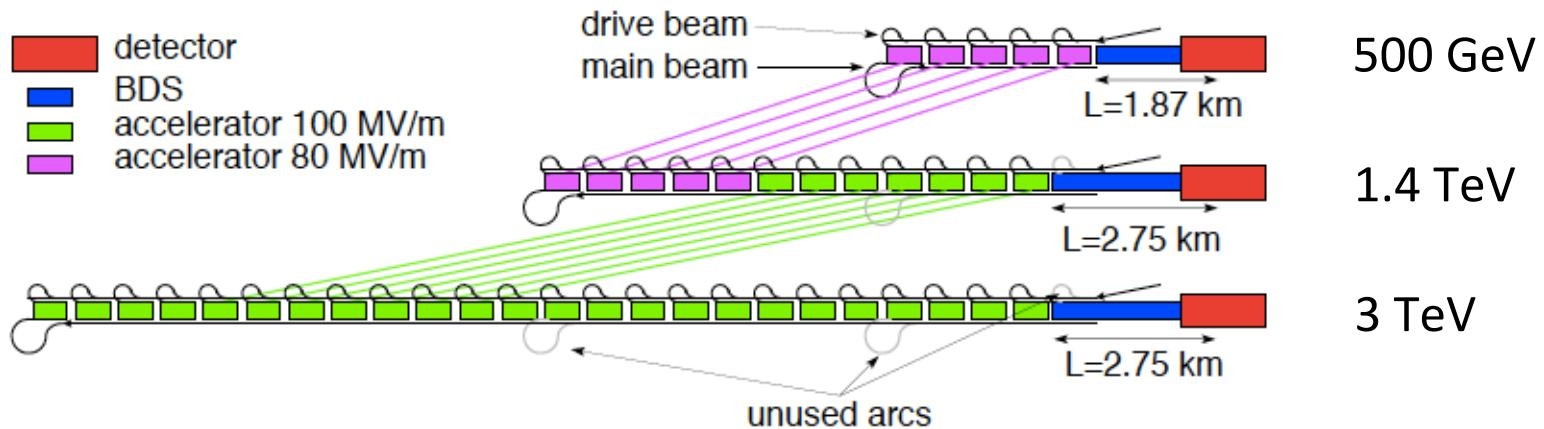
Fig. 3.5: Simplified upgrade scheme for CLIC staging scenario A. The coloured lines indicate the required movement of the modules from one stage to the next.
