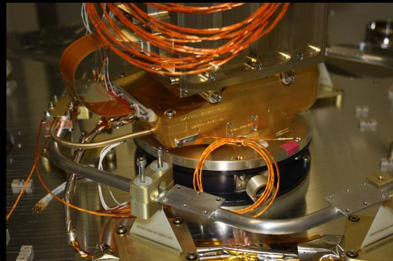
Preparation of Thermal Test with Heatpipe System
