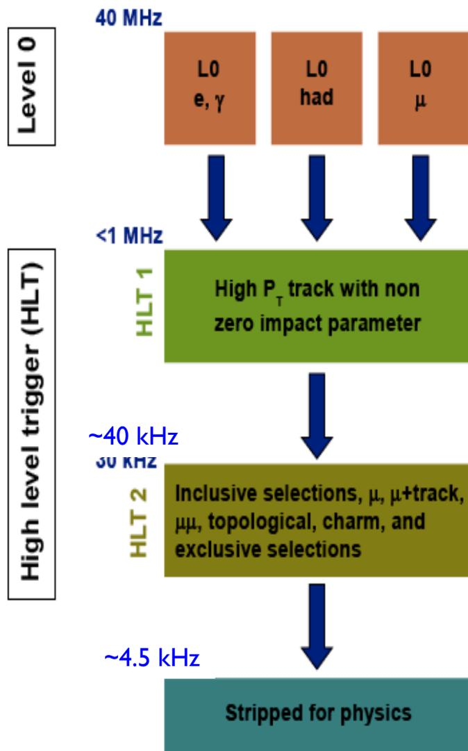
**Hardware level (L0)** 40 MHz of bunch crossing  $\rightarrow$  1MHz
