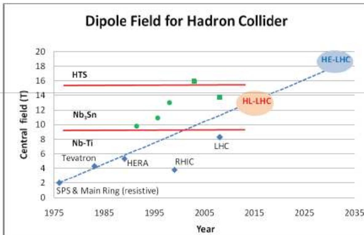
◆ Nb-Ti operating dipoles; ● Nb<sub>3</sub>Sn cos $\theta$  test dipoles ■ Nb<sub>3</sub>Sn block test dipoles
