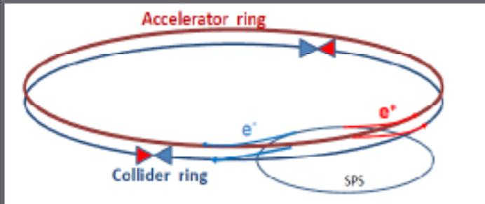
two ring scheme with top-up injection into collider ring
