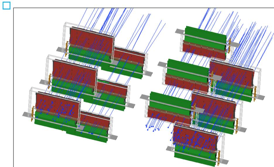
Ladder position in the Inner Tracker is known to 20  $\mu\text{m}$  precision
