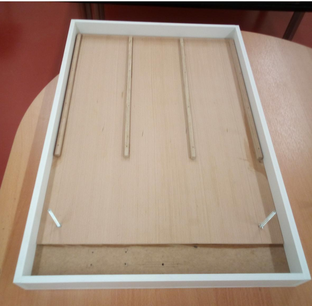
Detector enclosure from foam PVC 10mm
