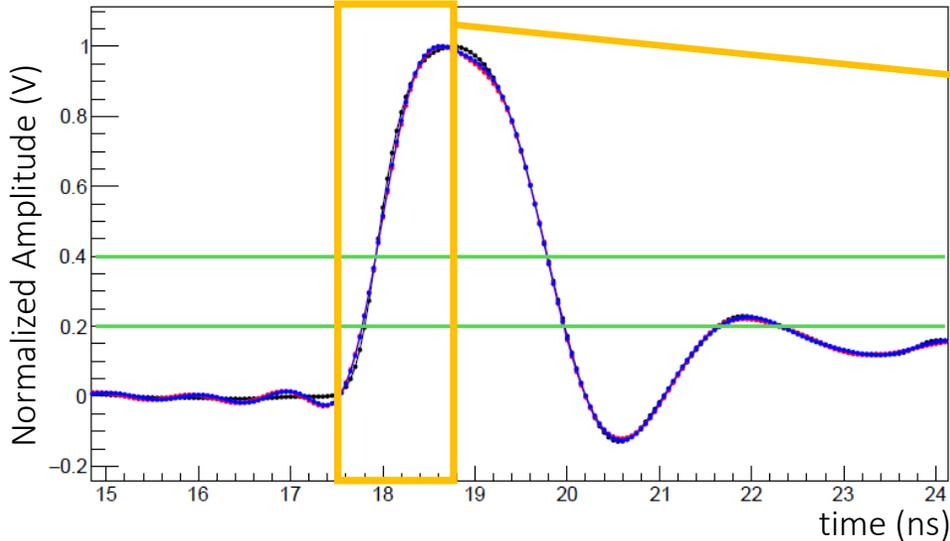
The leading edge of the waveform has large frequencies and the aforementioned cuts distort it and make less sharp. This results to a worse time resolution.
