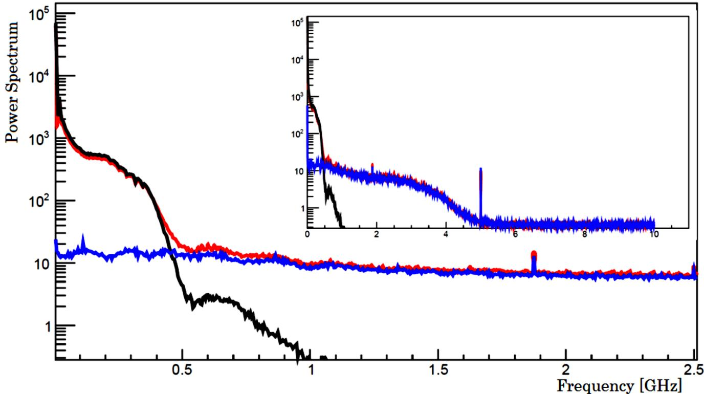
As the signal does not seem to have any dominant frequencies after 1GHz, the Fourier Filter can be applied as a lowpass filter with a cut in the region of 1-2GHz.
