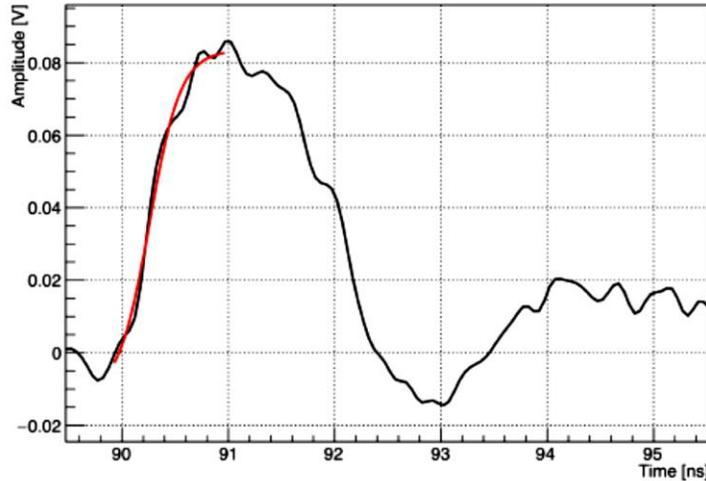
We tried different methods, including quadratic and cubic polynomial interpolation. We also tried to fit with the logistic and generalized logistic functions:
