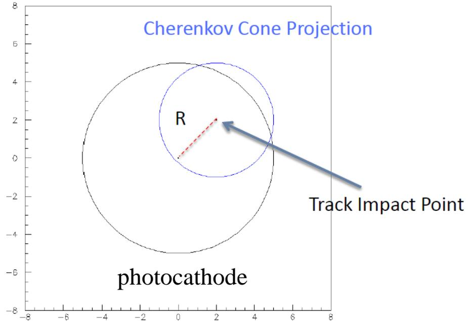
Every muon produces Cherenkov Photons whose population follows a Poisson distribution. However, not all the photons are deposited in the active area (photocathode). There exists a geometrical acceptance which describes the fraction of the accepted photons. Because it is a smooth function decreasing with the impact parameter, the center of the detector can be estimated.
