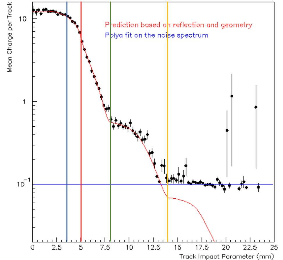
We used a toy Monte Carlo to find the geometrical acceptance using the geometry of the detector and a free parameter for the probability of reflection. By adjusting the probability of reflection we can describe the mean charge per track versus the impact parameter very nicely. The red line corresponds to the toy model, whilst the blue line to the background noise.
