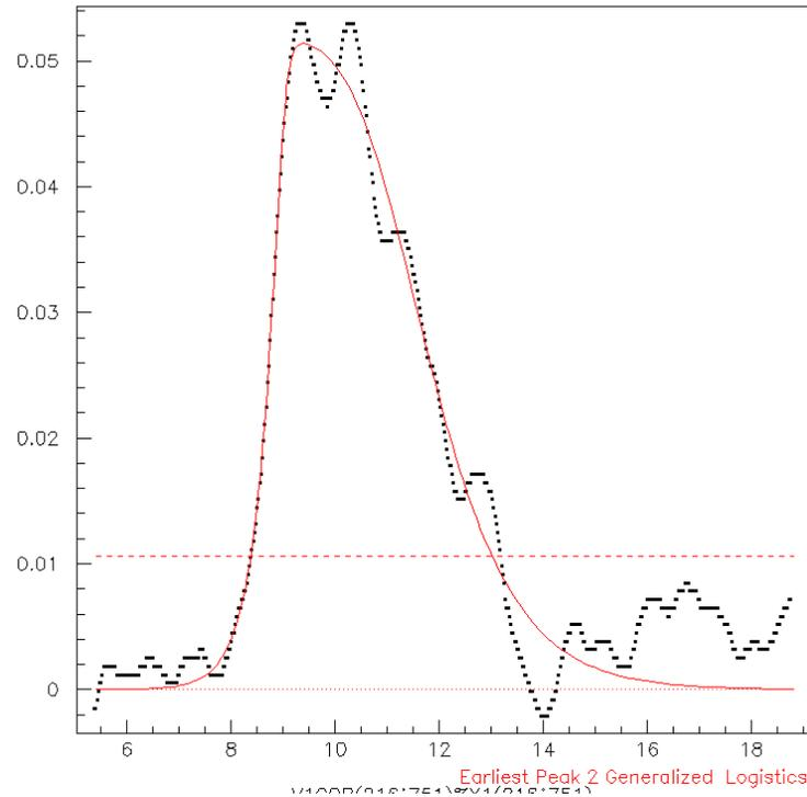
The e-peak charge was calculated by integrating the fit.
