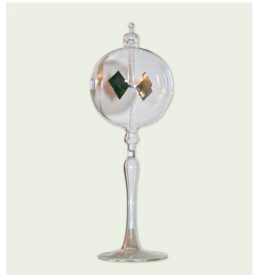
FIGURE 61 A commercial light mill turns against the light (Wikimedia).
