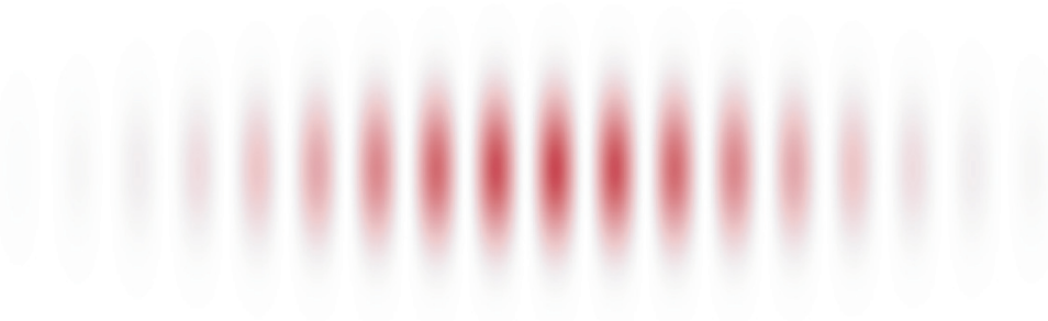
FIGURE 51 Two Gaussian beams interfering at an angle (© Rüdiger Paschotta).
