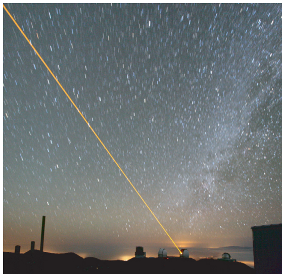
FIGURE 76 A sodium frequency laser beam is used as laser guide star to provide a signal for adaptive optics in large telescopes. The laser illuminates a layer of sodium found in the atmosphere at around 90 km of altitude, thus providing an artificial star. The images of the real stars are blurred due to the long exposure time of 3 min (photo Paul Hirst).
